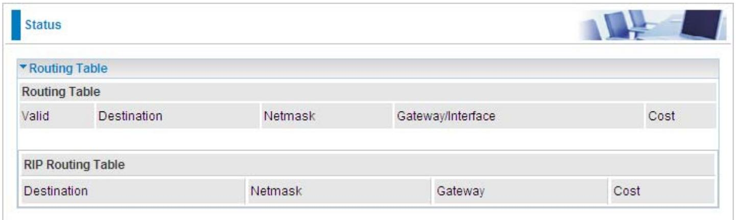
The screenshot shows a network configuration interface with a 'Status' tab. Underneath, there are two expandable sections: 'Routing Table' and 'RIP Routing Table'. The 'Routing Table' section contains a table with columns: Valid, Destination, Netmask, Gateway/Interface, and Cost. The 'RIP Routing Table' section contains a table with columns: Destination, Netmask, Gateway, and Cost. The interface also features a small image of a computer workstation in the top right corner.
