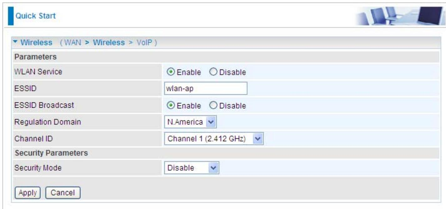
The screenshot shows a web-based configuration interface titled "Quick Start". The breadcrumb navigation is "WAN > Wireless > VoIP". The "Parameters" section includes:
