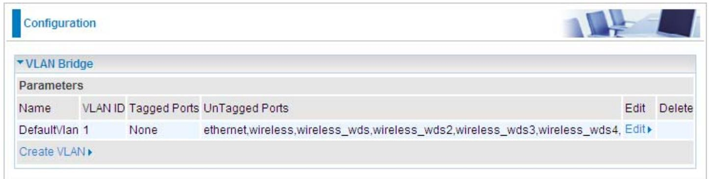
The screenshot shows a network configuration page with a 'Configuration' header. Below it is a 'VLAN Bridge' section. Under 'Parameters', there is a table with columns for Name, VLAN ID, Tagged Ports, UnTagged Ports, Edit, and Delete. The table contains one entry: 'DefaultVlan 1' with 'None' for Tagged Ports and 'ethernet,wireless,wireless\_wds,wireless\_wds2,wireless\_wds3,wireless\_wds4' for UnTagged Ports. Below the table is a 'Create VLAN' link.
