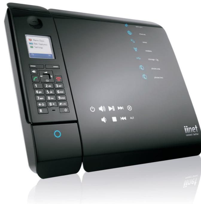
To display BoB2™ and the handset as one unit, they first need to be attached to each other. The handset will then get its charge from the BoB2™ USB port on the left hand side. This USB port is a dedicated charge port and not used for anything other than charging the handset. You will not need the power adapter that came with your handset so keep this in a safe place.
